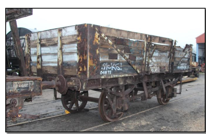
The nameplate on the wagon shows the number 118718. This tells us that it was designed and built in Swindon in 1931 for the Great Western Railway (GWR). Known as a "four wheel five plank open", it was one of the commonest types of wagon on the GWR and was used for carrying general merchandise or stone such as limestone or granite. When the railways were nationalised in 1948, it could have been used by British Railways anywhere in the country and
