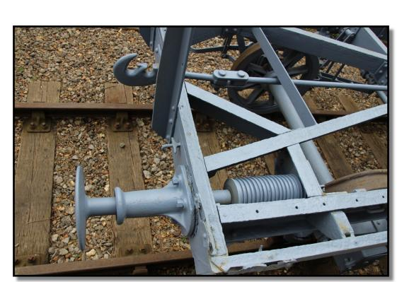
Also under the floor are four shock-absorbers, one for each of the four buffers.
