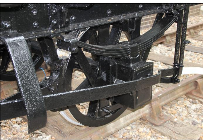
The first job was to paint the ironwork. We applied two undercoats and an additional rust-proofing coat where it was needed (especially under the floor) plus two black topcoats. Each coat took about 50 man-hours to apply, the detail of the wheel spokes being particularly fiddly. The paint is made to a special BR specification for rolling stock.
